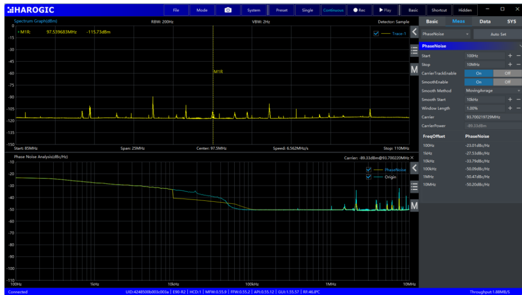
Figure 6 Phase noise analysis in SWP mode.
