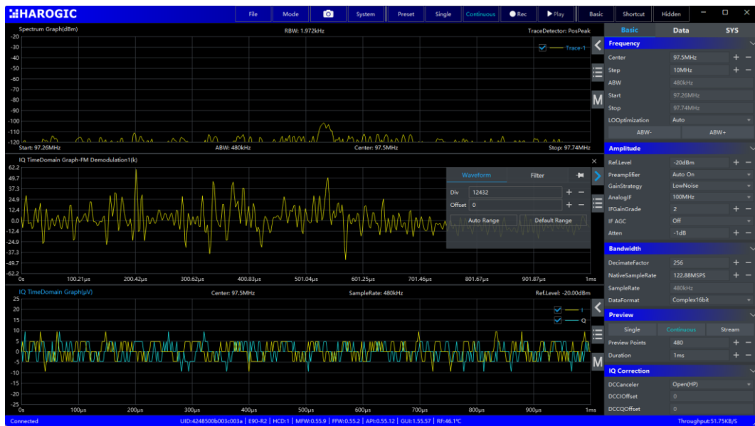
Figure 32 FM demodulation analysis in IQS mode.
